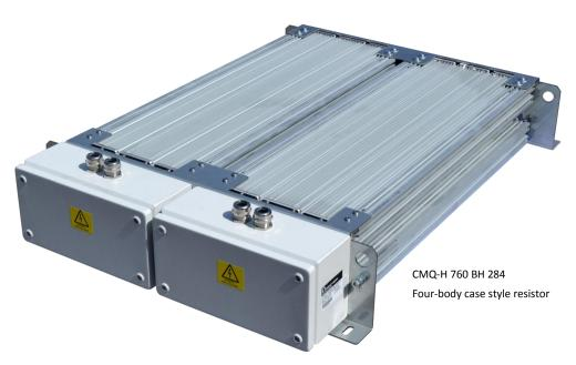
The CMQ-H and CMQ-V resistors with optional integrated thermal supervision from the Danotherm high power range of ALU-MINIUM-HOUSED COMPACT BRAKE ALPHA RESISTORS are electrically insulated compact resistors. They can easily be fitted into compact constructions and are especially designed to withstand high pulse-loads. The aluminium construction ensures that surface temperatures are kept low (see Table 3) such that any accumulated dust will not burn and trigger smoke alarms.
