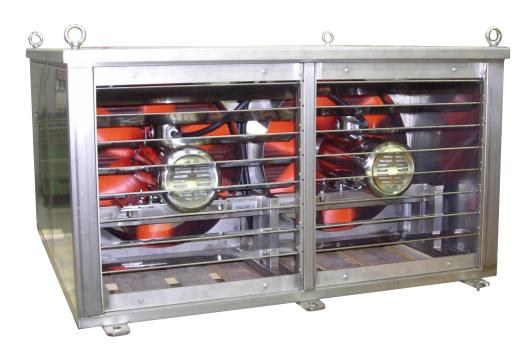
They are mainly used as brake resistor on top of cranes in harprotect the inside of the resistor unit when not in operation. bors. Two high power ventilators provide a strong air flow that cools a number of steel tube elements.
